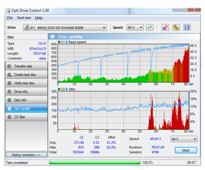
This is a scan of a low quality CD. There are some C2 errors at the 10 minute mark and a lot of C2 errors from the 55 minute mark.
