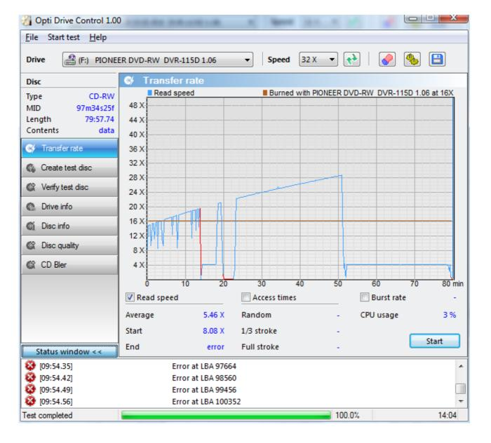
This screenshot shows the drive has a lot of trouble reading the disc. The drive slows down a lot, has to do many re-reads (visible as downward spikes) and cannot read certain parts of the disc (red lines).
