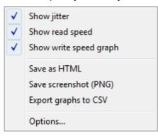
Show jitter: shows jitter line on the bottom graph if the drive can reports jitter
