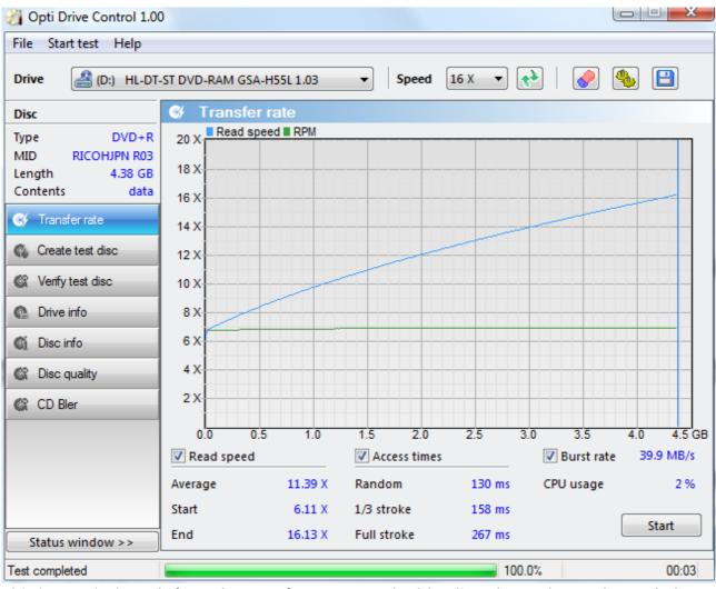
This is a typical result from the transfer rate test. The blue line shows the read speed, the green line shows the rotation speed in RPM.
